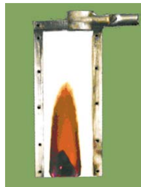
Fig. 1 Mostashari's flammability tester during the combustion. A low addition of flame-retardant was applied into the fabric, prior to the accomplishment of the flammability test
